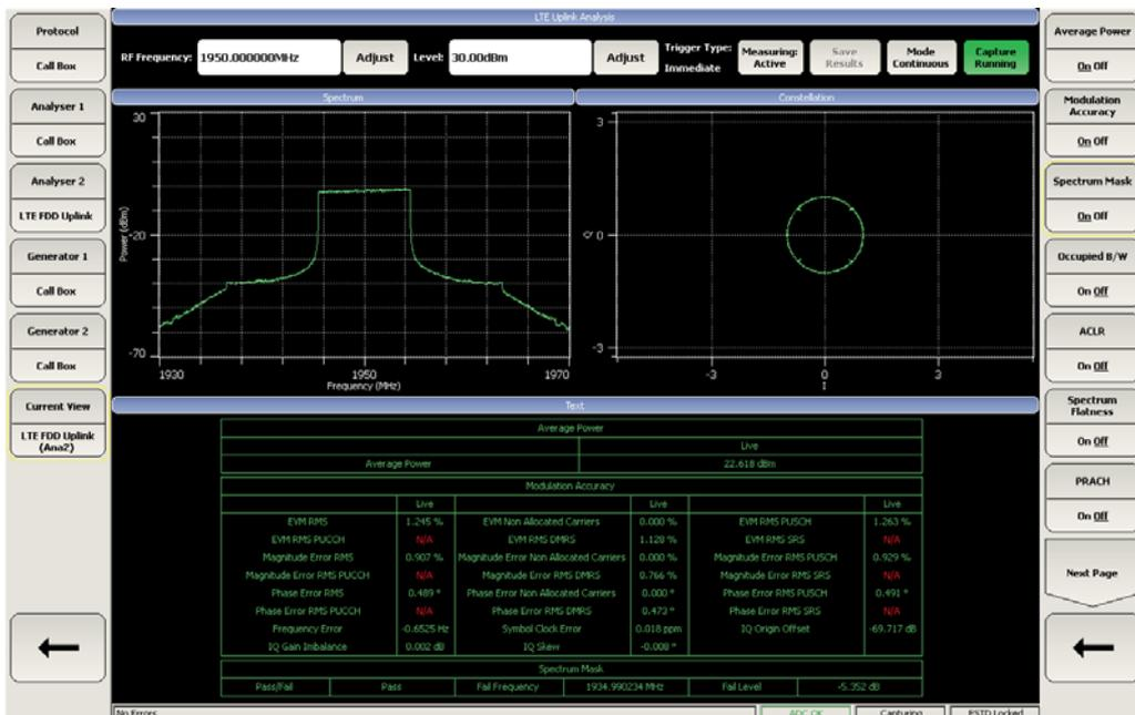
Figure 4. VSA/VSG LTE Measurements
