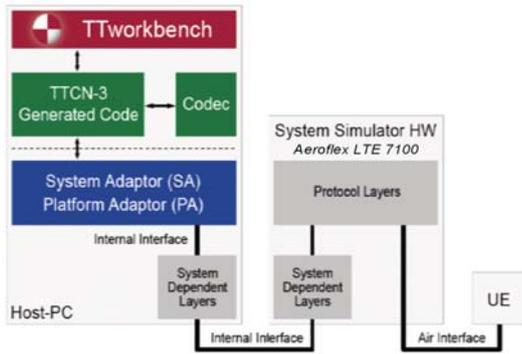
Figure 7. Aeroflex TTCN-3 Setup using 7100 Test Adapter
