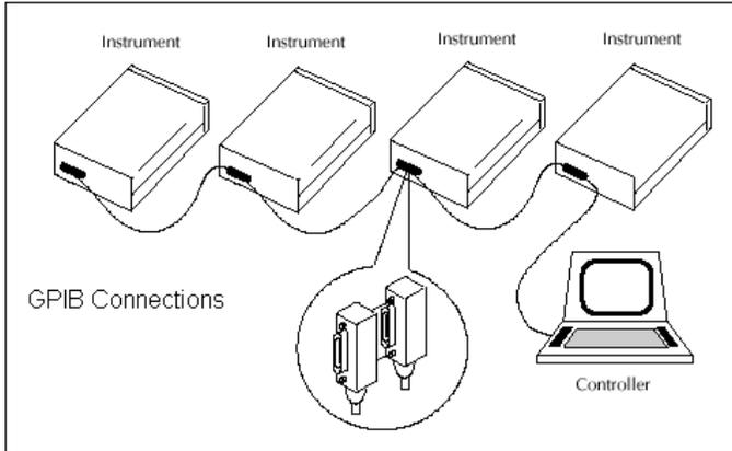
**Figure 1.** GPIB connections
